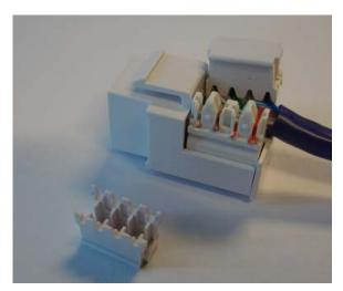
**Step 4.** Place the wire caps over each set of terminals and press down in place.
