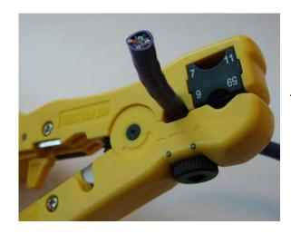
**Step 1.** Strip about 1" off of the outer jacket of the cable. If using Cat6 cable, trim off the spleen so that it doesn't get in the way of the wires.
