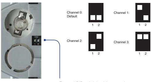
Exposed DIP switch bank between the battery slots.
