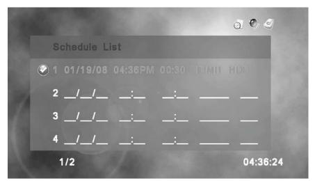
The Schedule List menu displays all scheduled recordings. Once a recording is complete, the entry is removed from the list. Scheduled recordings labeled with a  $\bigcirc$  are active recordings.
