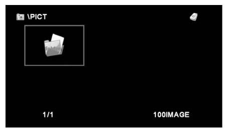
The Folder Menu displays the current folders located on the selected media. To change media type, press the HDD/SD button on the remote at any time. Use  $\blacklozenge$  and  $\blacklozenge$  to navigate the menu and press (in the selected folder.
