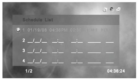
Once you have input all of the information for the recording it should already be set as active. To de-activate the recording for any reason, navigate to it using  $\blacklozenge$  and simply press the  $\blacktriangleright$  key on the remote. To re-activate it press  $\blacktriangleright$  again.
