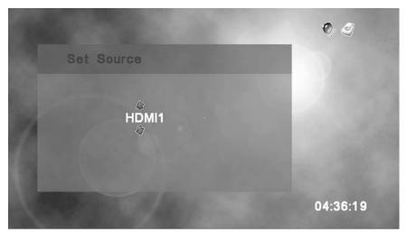
Set the input source for the recording using  $\clubsuit$  to select between HDMI1, HDMI2, COMPONENT or VIDEO. Press when you are done.
