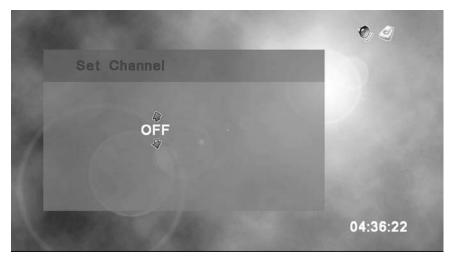
If the IR blaster is connected and set up, you can select a specific channel (up to 4 digits). Otherwsie, you should set to OFF mode when not using an IR blaster. Use  $\clubsuit$  to change each digit and  $\clubsuit$  to move between them. Once you have set the channel, press  $\overline{(\kappa)}$  to complete the Recording Setup.
