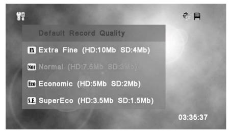
The default recording quality is set here. The table on the next page shows each recording option and its corresponding bit rate.
