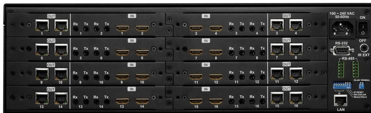
Figure 5-6 HIT-HDMI4K2KCAT5-X16416 Rear Panel for 16 Output/Input Jacks
